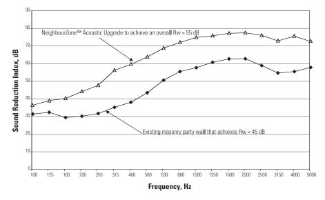
The graph on the left shows the improvement that will be achieved over various frequency bands<sup>2</sup>. The noise problems identified typically occur between the 250 Hz and 1000 Hz frequency bands. NeighbourZone<sup>™</sup> system NZ1 clearly meets the target 10 dB improvement in these frequencies (or subjectively halving the noise).
